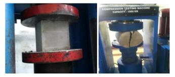
Fig. 1 Compression test (left) and splitting tensile test (right)
