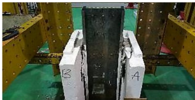
Figure-7. Failure mode of S4M14 test specimen
