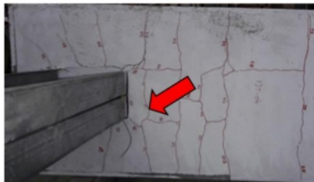
(c) IJT-06 first crack
