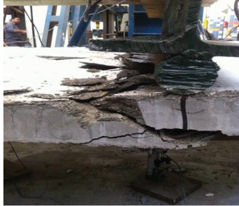
FIGURE 8. Transverse crack, CFS thickness 4mm
