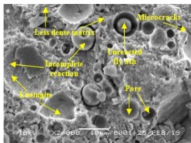
Fig. 24. Microstructure test results on mixed LGC at 20% kaolin and 14M NaOH
