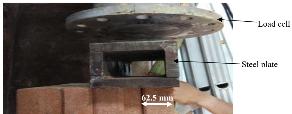
Figure 3: Eccentricity test set up
