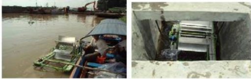
Figure 4: (a) Floating waterwheel on test on Musi River. (b) Floating waterwheel on test at sluice gate at Bangun Sari Village.
