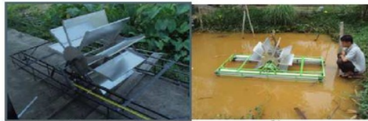
Figure 3: (a) The wheel and supporting frame in constructions. (b) The floating test is conducted with PVC pipes at the left and right sides.
