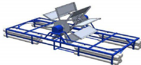
Fig. 2 Floating waterwheel with supporting PVC pipes on sides.
