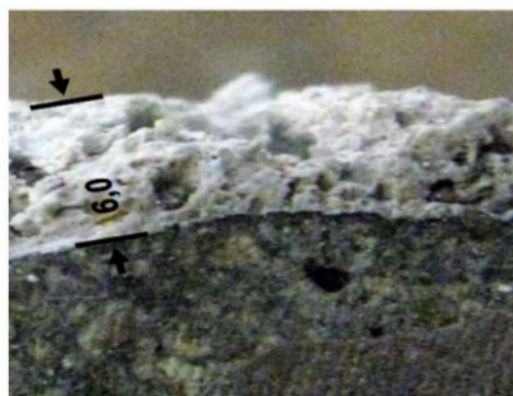
Fig 1. Sulfuric acid immersion concrete test results
