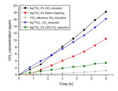
**Figure 7.** CH<sub>4</sub> concentration over time for the Ag/TiO<sub>2</sub> 2% sample in batch cleaning, and CO<sub>2</sub> reduction with Hg/Xe lamp and LED, as well as CO<sub>2</sub> reduction with metallic state  $Ag^0/TiO_2$  2%. Bare TiO<sub>2</sub> is used as a reference.
