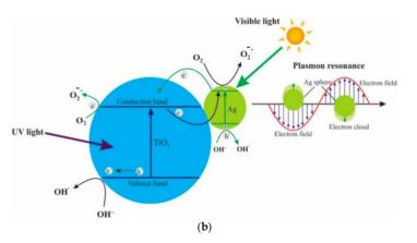
**Figure 2**. (a) UV-Visible spectra of  $TiO_2$  and  $Ag/TiO_2$  as pressed disks. Inset shows the material absorption magnification at 400–700 n; (b) surface plasmon resonance (SPR) effect of Ag species deposited on  $TiO_2$  surface, modified from reference [48].
