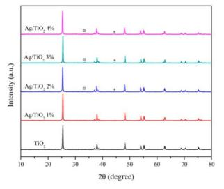
**Figure 1.** Powder XRD patterns of pristine TiO<sub>2</sub> and Ag/TiO<sub>2</sub> materials. Small squares ( $\Box$ ) at  $2\theta = 33.2^{\circ}$  indicate the presence of Ag<sup>I</sup> species and the small stars (\*) at  $2\theta = 44.4^{\circ}$  indicate the presence of Ag<sup>0</sup>.
