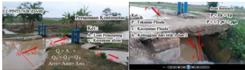
Figure 1 Video display explaining the concept of dynamic fluid and the Bernoulli principle on floodgates
