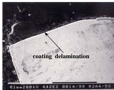
Figure 10.5 Sectioned of Tool A showing delamination of coating on the bevelled face after face milling for 5 seconds at 80 m/min
