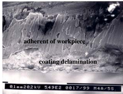
Figure 10.6 Delamination of coating and adherent of work material on Tool B after face milling for 5 seconds at 55 m/min
