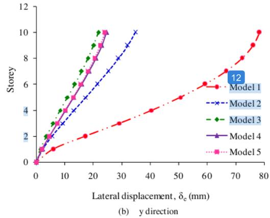
Fig. 5 Lateral displacements
