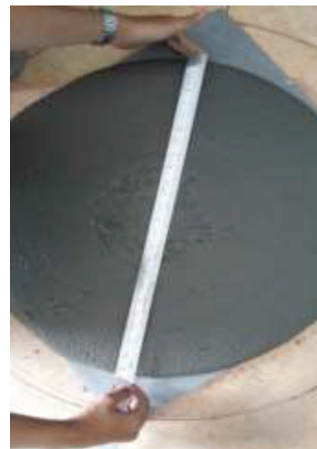
FIGURE 2. Slump flow test
