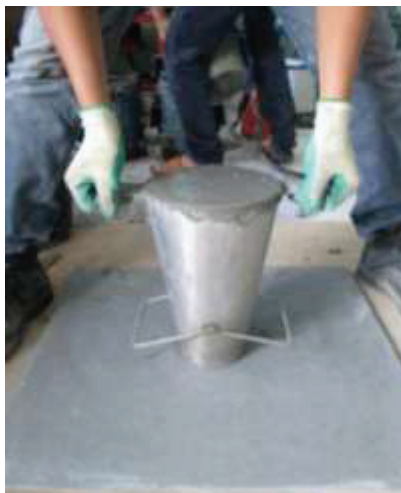
FIGURE 2. Slump flow test
