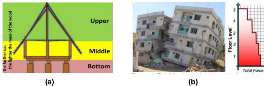
Figure 6. (a) Structure of Basemah House (modified from Rinaldi et al., 2015) and (b) Destroyed building Caused by Earthquake (Murty, 2005)
