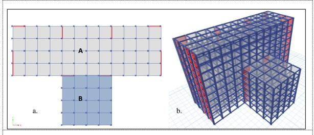
Figure 17. Model 4A (after shear walls were installed): a) the plan, b) 3D.
