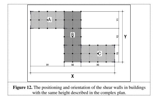
• With the formulas below, calculate the proportional shear wall area of each block. Blocks with larger plans also have larger shear walls and vice versa:
