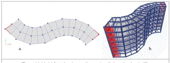
Figure 16. Model 3A (after shear walls were installed): a) the plan, b) 3D.
