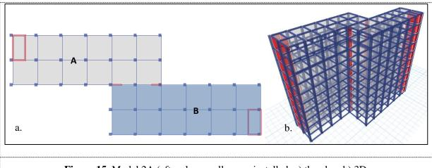
Figure 15. Model 2A (after shear walls were installed: a) the plan, b) 3D.
