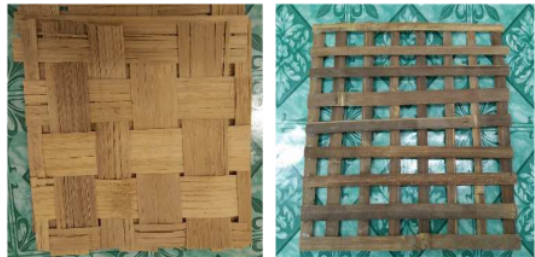
(b) Woven bamboo Fig. 2 Reinforcement
