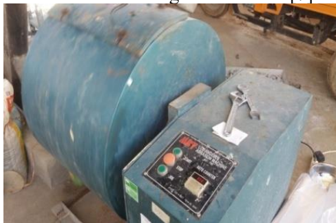
figure 3. Cantrabro test with Los Angeles machine
