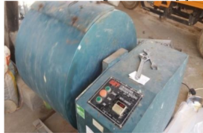
figure 3. Cantrabro test with Los Angeles machine
