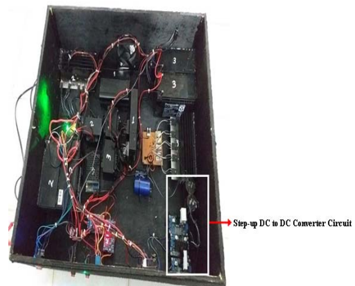
Fig. 4. Results of the Design of the Circuit of Step Up DC To DC Converter in box 2 on the block diagram of Fig. 1.
