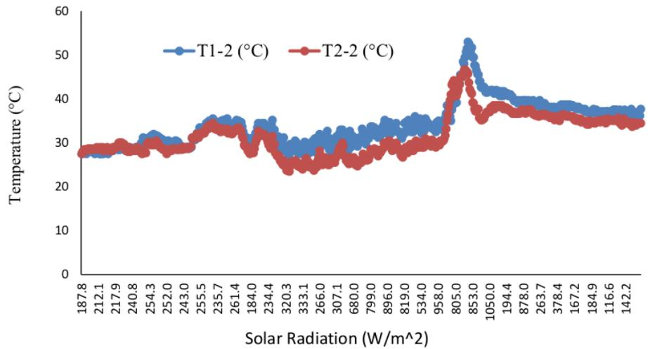
**Figure 4.** Comparison between the below surface temperature of the PV panel using perforated plate cooler (T1-2) and without perforated plate cooler (T2-2) on 4 February 2020
