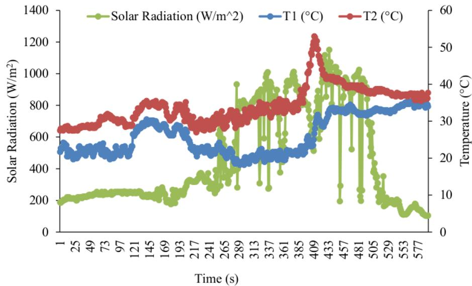
**Figure 3.** Comparison between PV panel surface temperature using perforated plate cooler (T1), PV panel surface temperature without cooler (T2) and solar radiation on February 4, 2020
