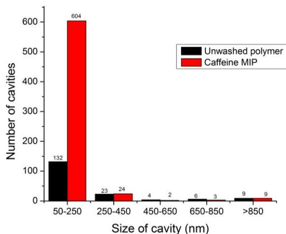
Fig. 4. Number of cavity size distributions of unwashed polymer and caffeine MIP.
