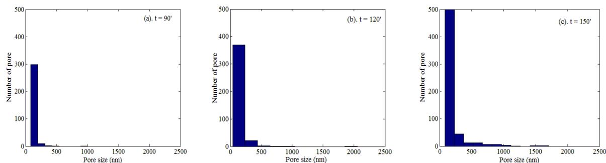
Fig. 3. Histograms of pore size distribution of atrazine-based MIPs produced by the heating times of (a) 90, (b) 120, and (c) 150 min.
