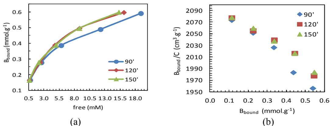
Fig. 4. Binding isotherm or saturation binding curves. (a)  $B_{bound}$  of atrazine against free concentration and (b) Scatchard plots between bound concentration/ initial concentration against bound concentration.
