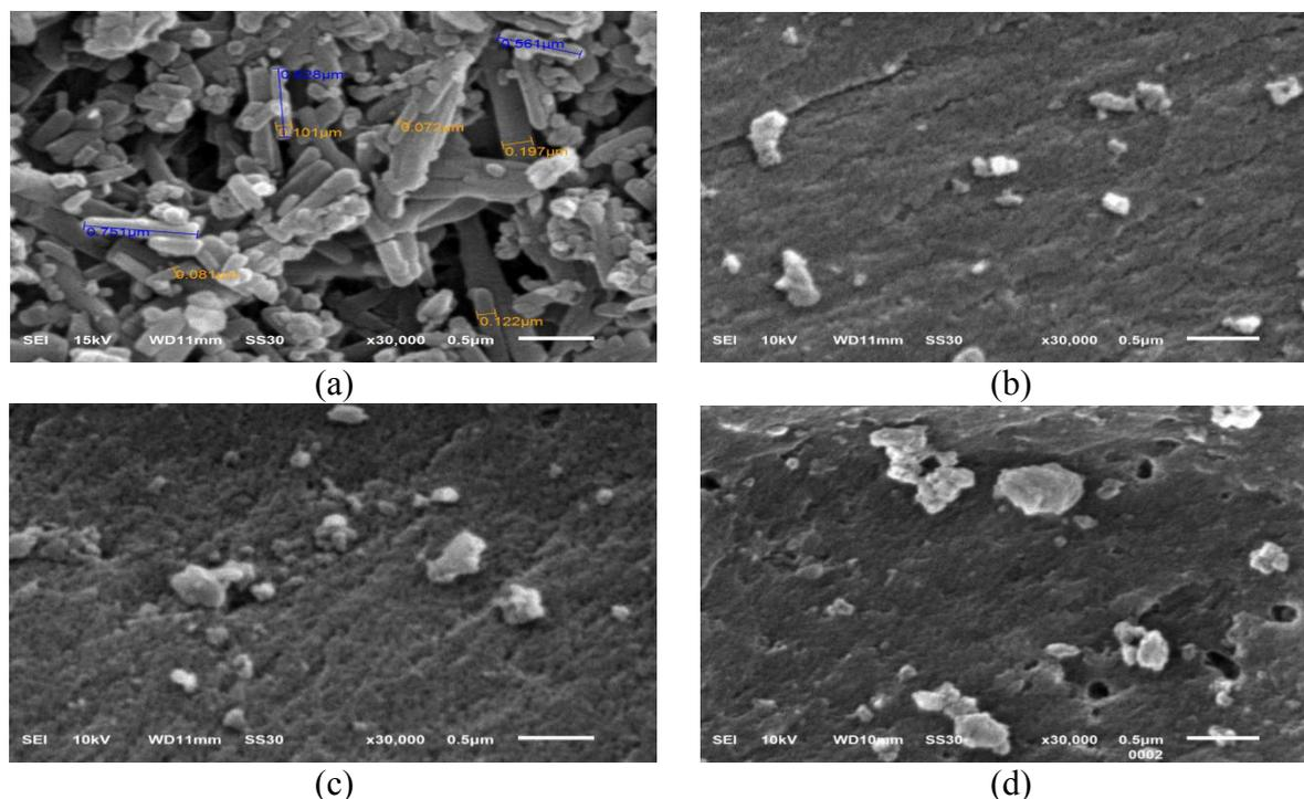
Fig. 2. SEM images of (a) atrazine standard and atrazine-based MIPs produced by heating times of (b) 90, (c) 120, and (d) 150 min.
