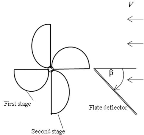
Fig. 4. Top view of Savonius rotor
