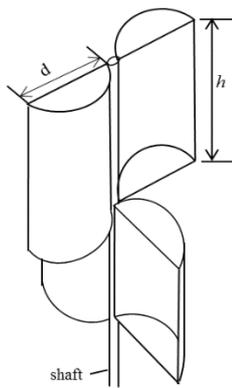
Fig. 2. Savonius turbine
