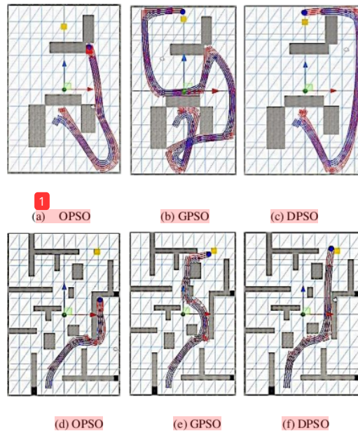
■ = Target ■ = Static Obstacles Fig. 3. Trajectory control with static obstacle in cluttered environment
