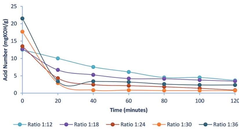
Figure 5. Effect of esterification time on acid number by various oil to methanol ratio
