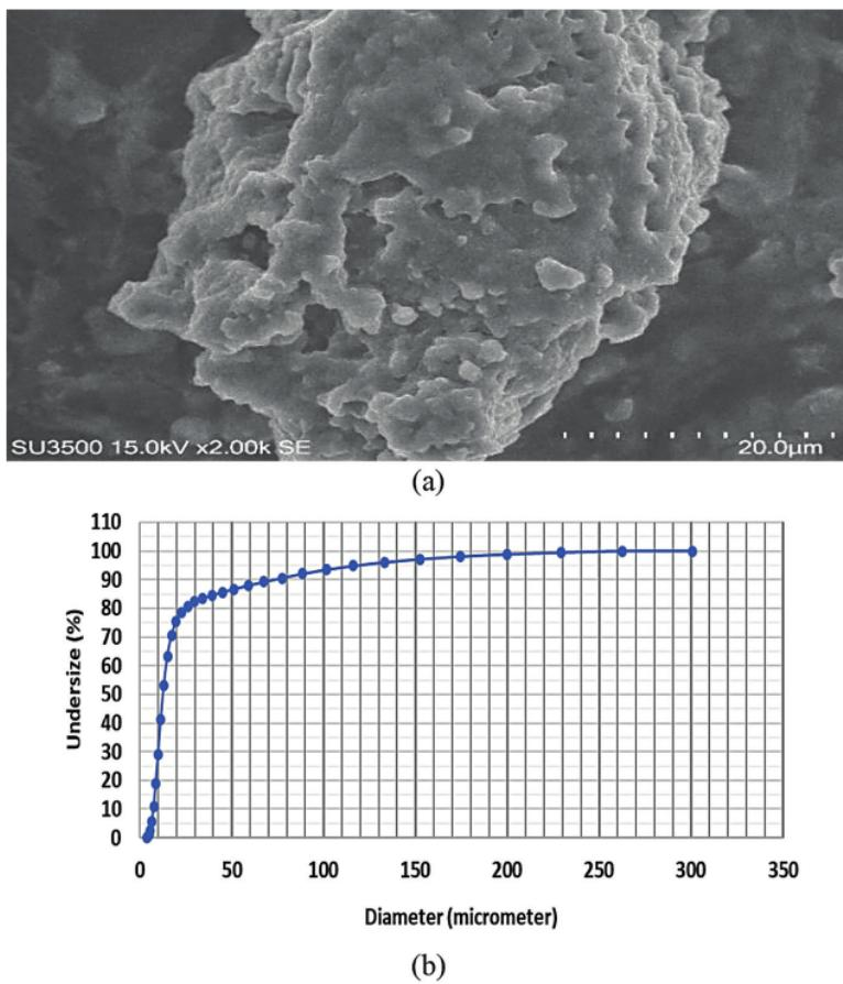
**Figure 3.** (a) SEM image of hydrotalcite at 2000 times of magnification
