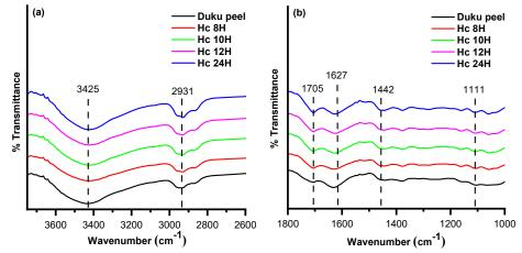
**Fig 3.** FTIR spectra of Duku peel and Hc at 200 °C in different times of hydrothermal process at wavenumber (a) 2600–3750 cm<sup>-1</sup> and (b) 1000–1800 cm<sup>-1</sup>
