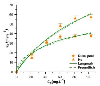
**Fig 7.** Effect of concentration and temperature on the adsorption of Cr(VI) onto Duku peel and Hc
