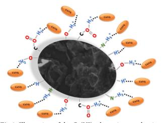
Fig 9. Illustration of the Cr(VI) adsorption mechanism
