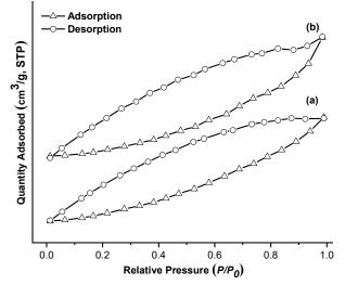
Fig 4.  $N_2$  adsorption-desorption isotherm of the (a) Duku peel and (b) Hc
