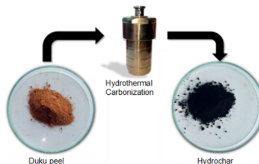
Fig 1. Schematic illustration of hydrochar formation using hydrothermal carbonization method
