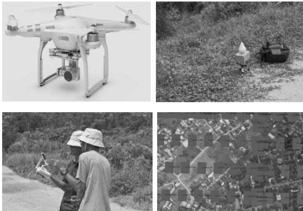
Figure 2. The UAV, marker point (GCP) and GPS RTK used in the study and the illustration of the process of acquisition and data processing
