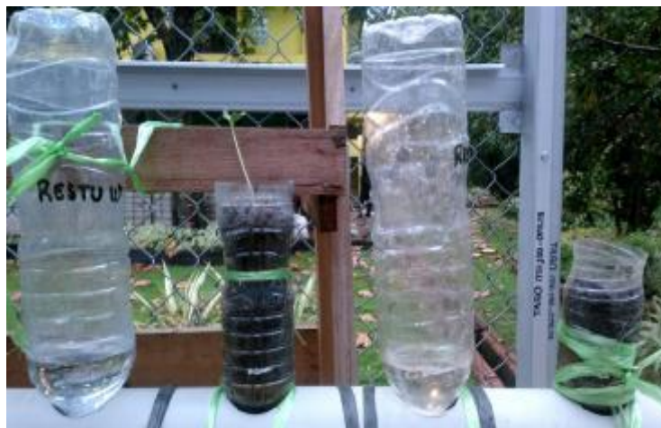
Figure 2. Experimental application of groundwater depth to supply irrigation water to the crop
