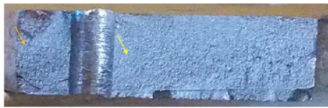
Figure 4. Fracture surface on the specimen with SDH 2.5 mm
