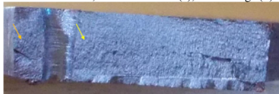
Figure 6. Fracture surface on the specimen with SDH 3.0 mm
