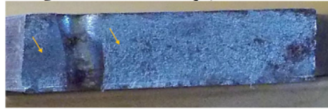
Figure 2. Fracture surface on the specimen with SDH 2.0 mm
