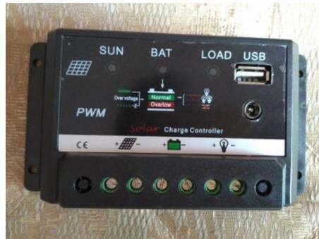
Gambar 2. 13 *Solar Charge Controller*
