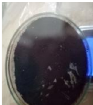
Figure 1. The Fe-Al metal milling results
