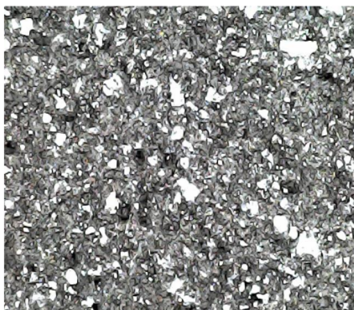
Figure 2. Microscopy Capture Using Digital Microscope of Ti-Co/Dots 50:50 Spraying Method Surface
