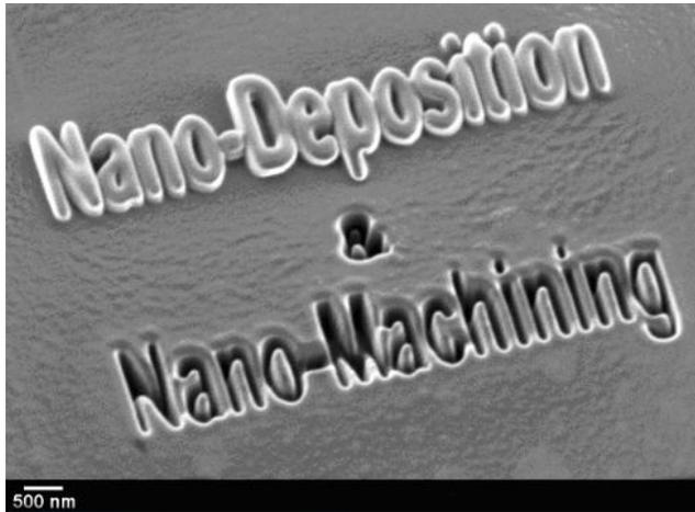
Gambar 21 Nano Depositioning dan Nano Mahining
