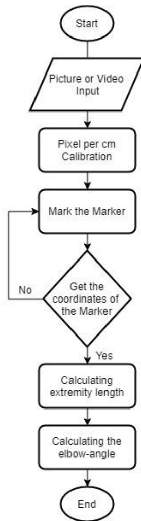
Figure 5. Calculation of elbow angle software Flowchart
