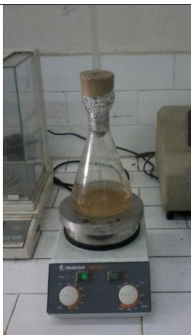
Refluks of solid using 150 ml  $\text{H}_2\text{SO}_4$  1 N
