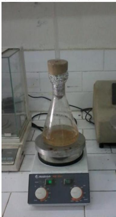
Refluks of sample by using 150 ml aquadest
