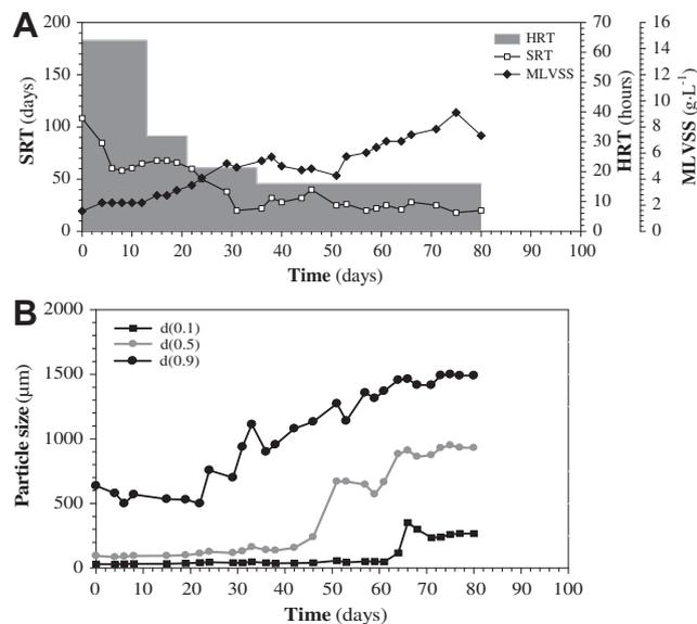
**Fig. 3** – The SBR operation hydraulic retention times (HRT), sludge retention times (SRT) and mixed liquor volatile suspended solids (MLVSS) (A). Sludge particle size distribution during the SBR operation for granule formation (B). The filled black circles are the 90th percentile size (i.e. 90% of the sludge is smaller than that value), the filled grey circles and the filled black squares are 50th and 10th percentiles of the particle sizes respectively.
