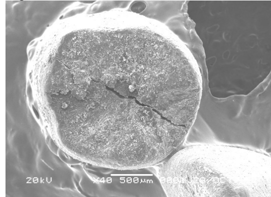
Figure 4. Scanning electron micrograph of fracture surface IR 64 variety.
