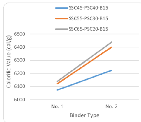
Fig.6. The effect of binder type on calorific value of briquette (cal/g) at various compositions
