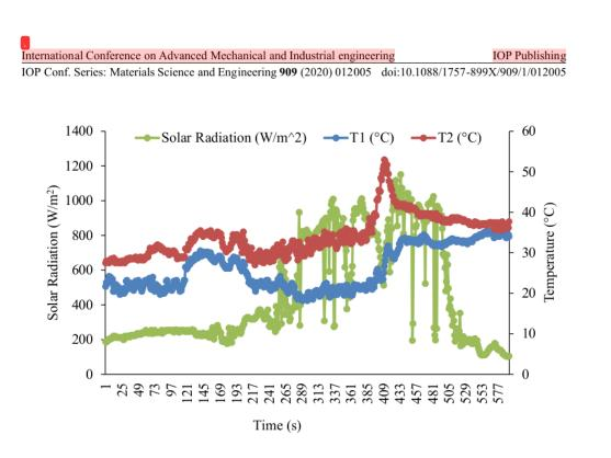
**Figure 3.** Comparison between PV panel surface temperature using perforated plate cooler (T1), PV panel surface temperature without cooler (T2) and solar radiation on February 4, 2020
