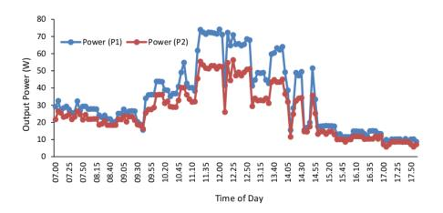
Figure 5. Comparison between PV panel output power using perforated plate cooler (P1) and PV panel output power without cooler (P2) on February 4, 2020
