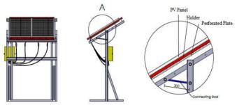
Figure 1. Structure of PV panels and perforated plates being tested
