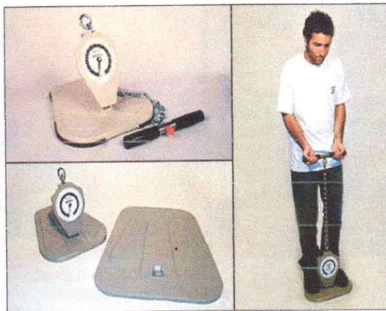
Gambar 2.6 Back and leg dynamometer.
