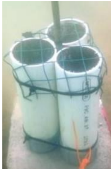
Figure 2. Modified sediment trap design (Windusari et al., 2015)
