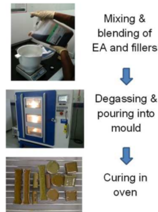
Fig. 1 Aluminium filled epoxy preparation with filled metals
