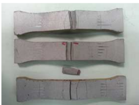
Fig. 9 Visible cracks after compression tests
