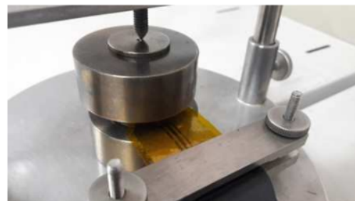
Fig. 2 Kapton® insulated sensor in between \phi 30 mm disc samples
