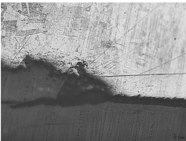
Fig. 14. Cracks start from corrosion pits.
