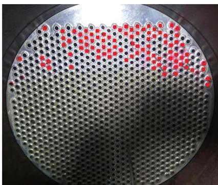
Fig. 2. Deposits of material-clogged SS 304 tubes on the top side
