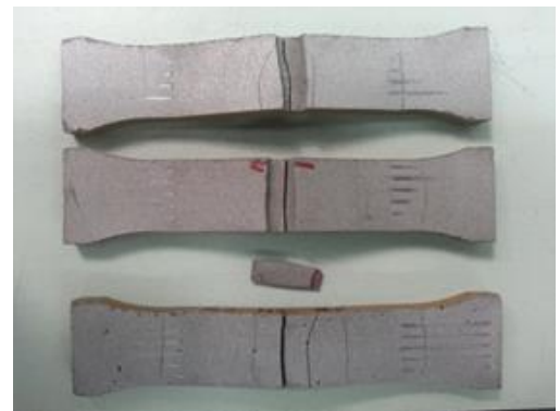
Fig.6. Visible cracks after compression tests
