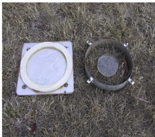
Figure 1. Instrument for soil respiration measurement consists of Perspex lid, metal ring and dish containing 0.5 M KOH. (Photo courtesy of Tongway and Ludwig, 1996).
