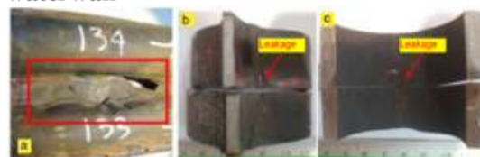
Figure 7. Visual Inspection of Waterwall Tube Boiler Failure.
