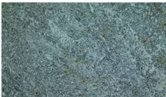
Figure 9. Micro Structure of Water Wall Tub at location 1 - Welding metal with 500X magnification
