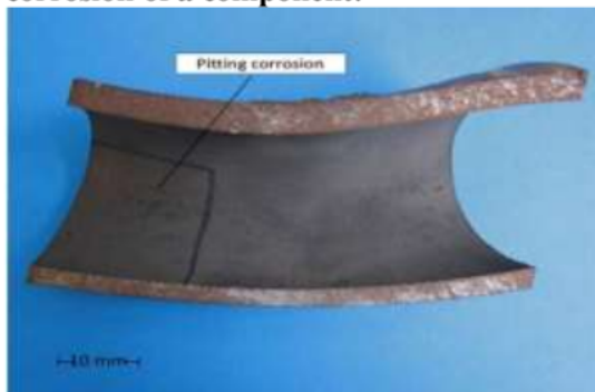
Figure 1. Pitting Corrosion (Duarte et al., 2017)
