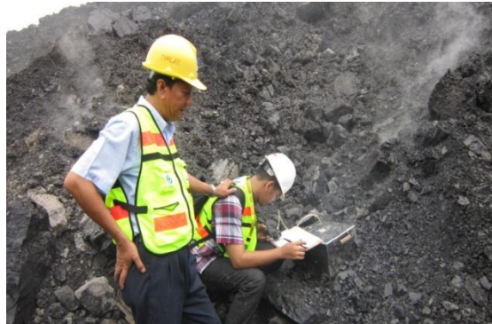
Figure 1 Measuring the Emission of CH 4 at the Front of Mine
