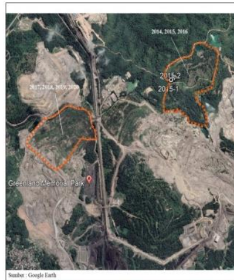
Figure 1. Aerial view of Banko Barat coal mine area showing different years of revegetation. The dotted red lines indicate current boundary of reclamation. The gray area indicates the former pit of coal reserves.
