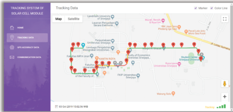
Figure 21.15 Visualization of coordinate data and the signal strength in real-time test of tracking system
