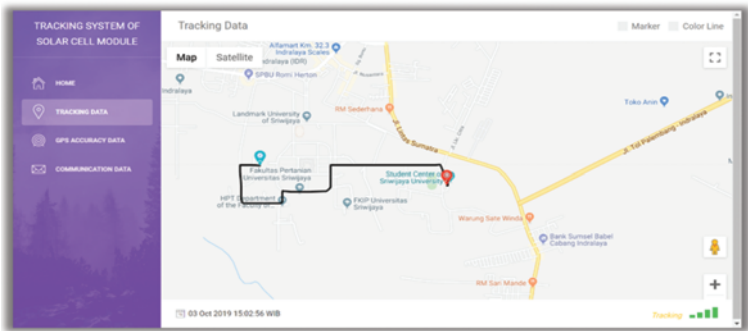
Figure 21.14 System interface in tracking mode
